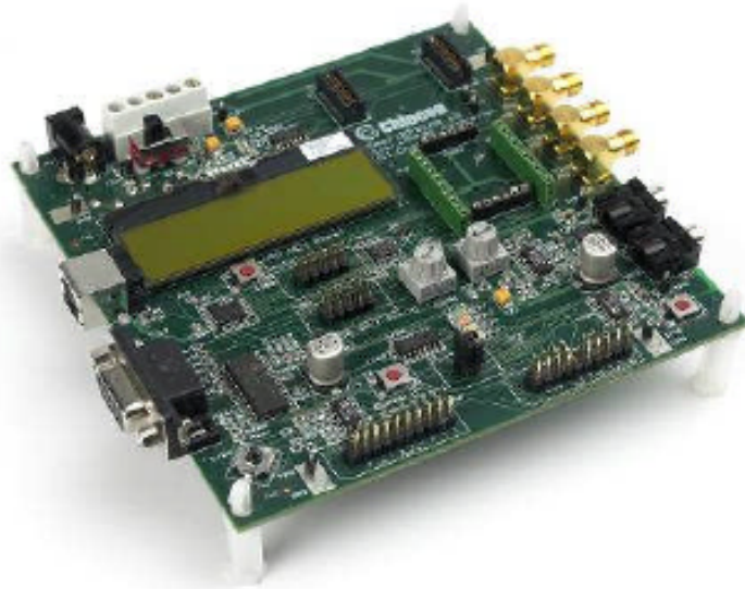
(b) SmartRF04EB evaluation board used in our implementation.
